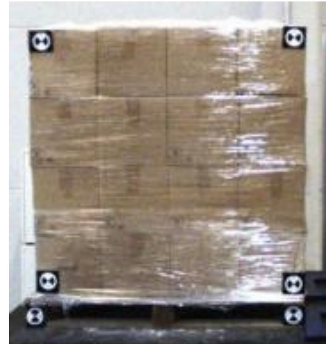
Stability tests: 4 targets, 1 per corner Tilt tests: 2 targets, pallet base corners
