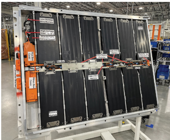
An example of the current ID.4 battery pack on display in the Chattanooga pack-assembly plant. This 82 kWh pack uses LG-supplied NCM712 cells and weighs 493 lb. A new pack using SKI-supplied NCM811 cells recently entered production.
