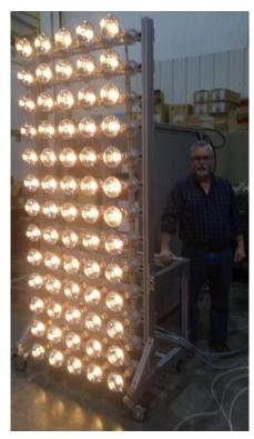
Portable or permanent array designs with movement are available. Fully automated operator interface controls irradiance, lamp zones, and other test variables.
