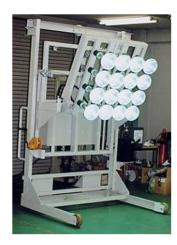
Portable or permanent array designs with movement are available. Fully automated operator interface controls irradiance, lamp zones, and other test variables such as diurnal cycle.
