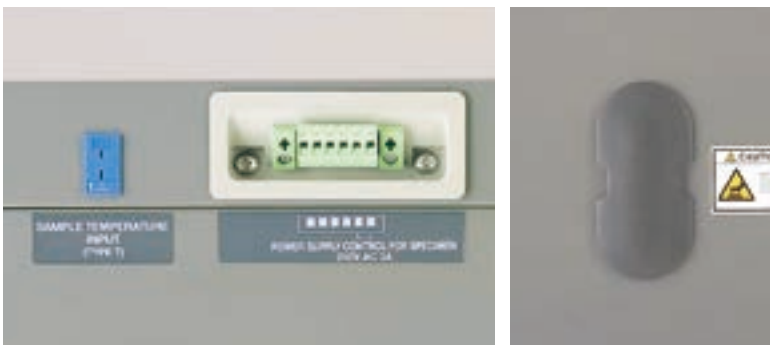
Specimen temperature input terminal (Left) Specimen power supply control terminal (Right)
