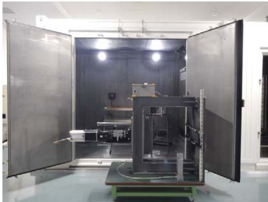
Figure 5. Equipment for conducting nail penetration test at controlled environmental temperatures (Made by ESPEC; installed in ESPEC's Battery Safety Testing Center.)
