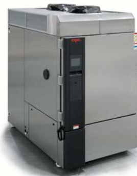
Air-cooled condenser on top of the chamber saves utility and installation cost. Adds 350mm (14") to the exterior height.
